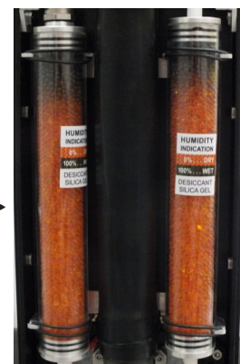
Silica gel desiccants in the fixture arm
