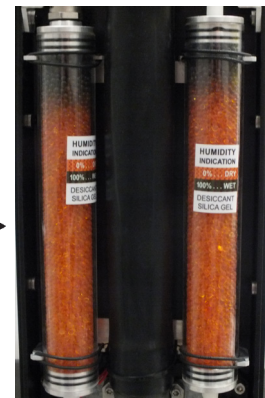
Silica gel desiccants in the fixture arm
