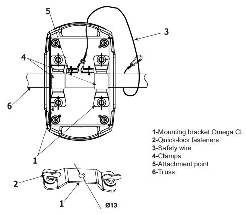
When installing fixtures side-by-side, avoid illuminating one fixture with another!
