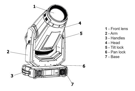
The head has to be locked for transportation- the tilt lock latch (5) and the pan lock latch (6) have to be in the locked positions. To unlock the head, move these latches to unlock positions before operating the fixture.
