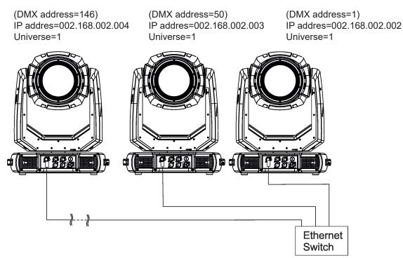
An advised PC setting: IP address: 002.xxx.xxx / 010.xxx.xxx (Different from fixture IP addresses) NET mask: 255.0.0.0
