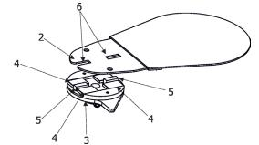
4. Place a new frost module into the frost holder (3). Check, that both slots (6) snapped correctly into two protrusions (5) in the holder (3).
