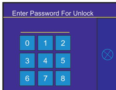
Enter the default password (5242) to enter the main menu of the FollowSpot Controller. The password prevents unauthorized person from changing setting of the FollowSpot Controller (password can be changed or switched off via the menu Settings).
