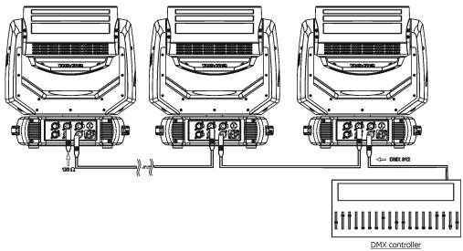
Connect the DMX-output of the first fixture in the DMX-chain with the DMX-input of the next fixture. Always connect one output with the input of the next fixture until all fixtures are connected. Up to 32 fixtures can be connected.
