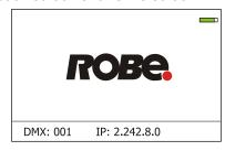
Note: The green icon at the top right corner of the screen indicates the level of the display battery charging. If the whole icon is green, the battery is fully charged while the red icon indicates exhausted battery. The battery charges during fixture operation, its charging lasts cca 6 hours.
