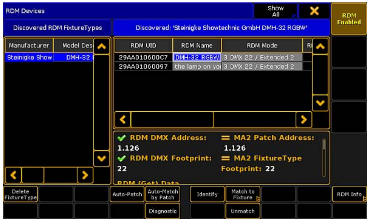
Auto-patched RDM fixture
