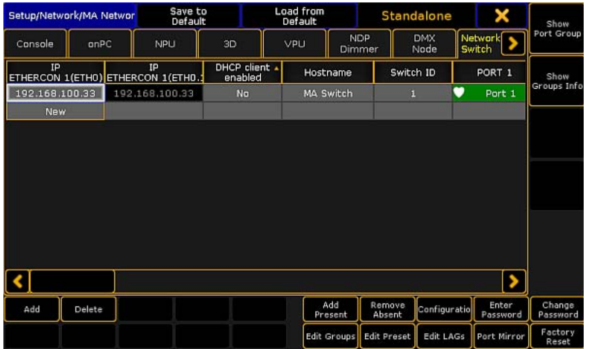
MA Network Configuration - Network Switch
