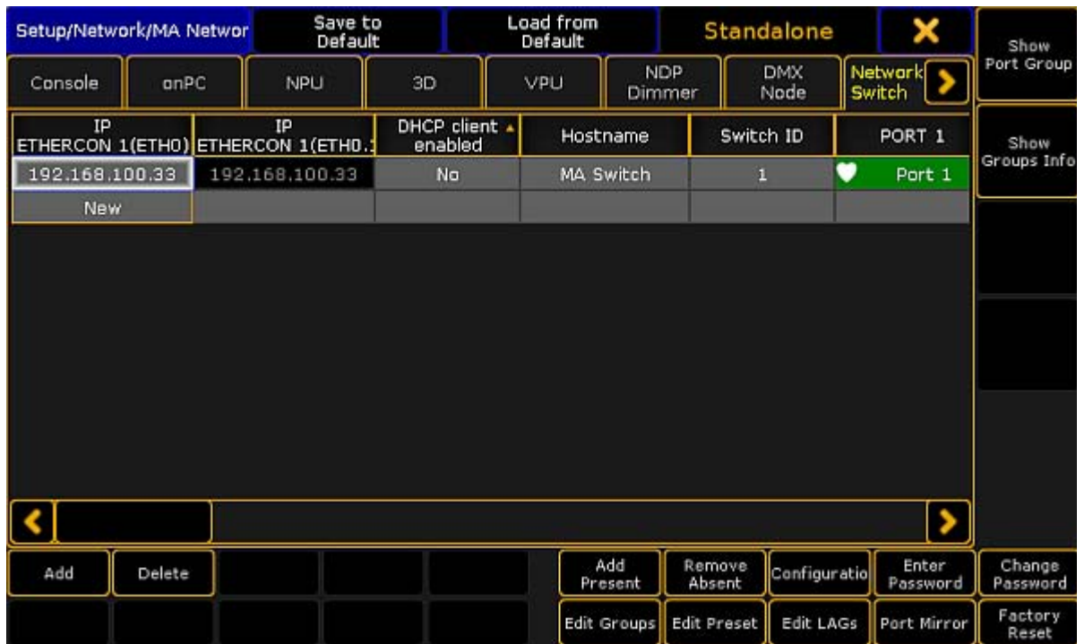
MA Network Configuration - Network Switch
