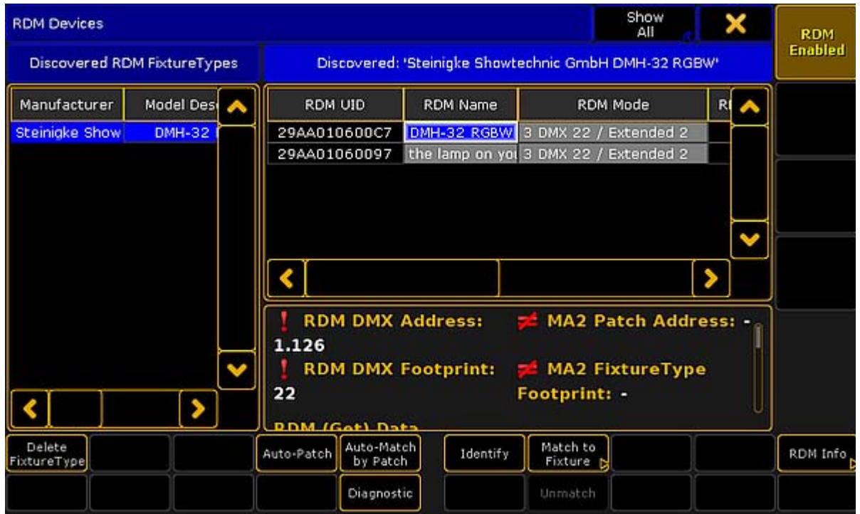
Setup - patch & fixture schedule - RDM devices
