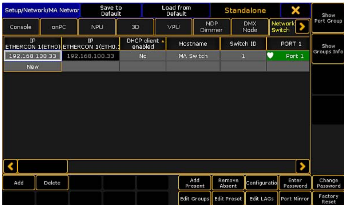
MA Network Configuration - Network Switch
